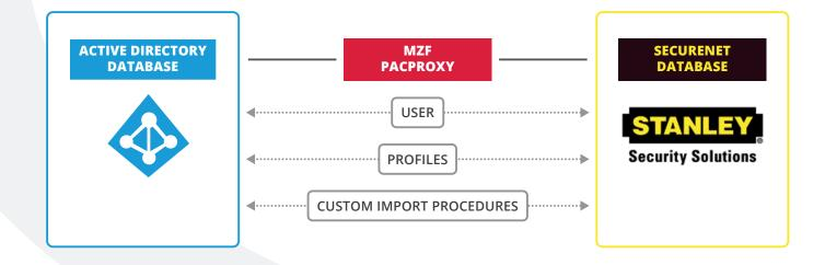
The metaSEC PSN Active Directory Connector is an add-on for the Stanley PAC SecureNet and delivers a solution for synchronizing the keyholder database with the central user database in Microsoft Windows based network.
